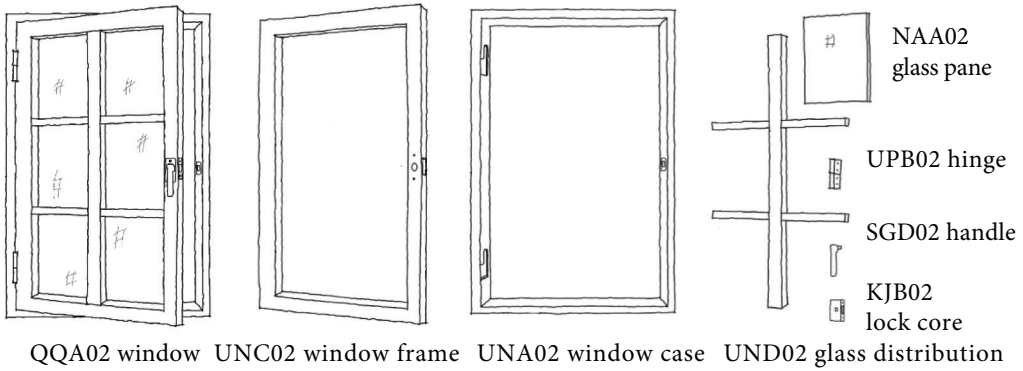
Figure 6. (Eckerberg, 2019) Example of an integral component consisting of separate components
